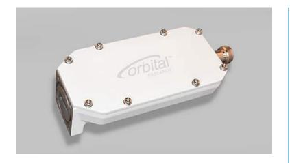
This entry-level Ku-band Phase Lock Loop (PLL) LNB is enhanced to meet customer-specific requirements. It offers extended bandwidth of up to 1050 MHz with 40 to 60 dB gain – and is customizable for wideband applications between 10.70 GHz and 12.75 GHz. The LNB provides excellent performance for consumer video and broadband applications, as well as DVB-2 and DVB-2X waveforms.
