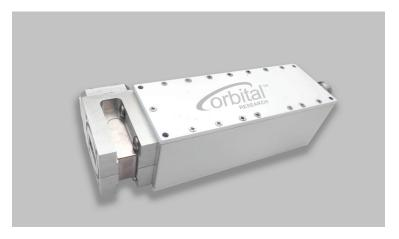
This Ku-band LNB is tuned to the exact frequency you require. It provides user bandwidth of up to 1.05 GHz in the 10.7 GHz to 12.75 GHz range – and offers exceptional performance for both commercial and military satellite communication (SATCOM) applications. 2.05 GHz wideband output versions are also available.
