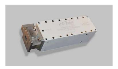
Our Ku-band low noise block downconverter (LNB) with multiple local oscillators is built for terrestrial and airborne satellite terminals. It lets you switch between different Ku frequency bands in the 10.7 GHz to 12.75 GHz range – and offers 1.05 GHz of bandwidth per LO. This LNB makes it possible to support several services with the same hardware.
