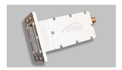
This external reference C-band LNB delivers excellent phase noise and local oscillator (LO) stability. It operates from 3.40 to 4.20 GHz, provides 60 dB of gain and delivers a noise temperature of 25K. Built for professional SATCOM and available in 500, 600 and 800 MHz bandwidths, this high-quality off-the-shelf LNB is perfect for most C-band applications – particularly where rain fade is a concern.
