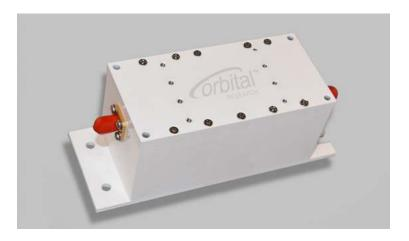
Orbital Ka-Band Block Downconverters (BDCs) with Fixed Local Oscillators provide bandwidth of up to 1 GHz and can be tuned anywhere in the following Ka frequency bands: 18.2 to 20.2 GHz and 20.2 to 22.2 GHz. These BDCs deliver superior performance for broadband Ka satellite communications – and their flat frequency response supports high data rate applications with very low bit error rates (BER).
