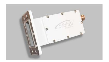
This external reference C-band LNB is enhanced to meet demanding specifications such as superior gain flatness, local oscillator (LO) stability and VSWR. The unit provides bandwidth of up to 800 MHz in the 3.40 to 4.20 GHz frequency range – and offers options like temperature-compensated gain and gain variations between 40 and 60 dB. This LNB is built for commercial and military SATCOM applications and is a great choice to help mitigate rain fade in temperate regions.
