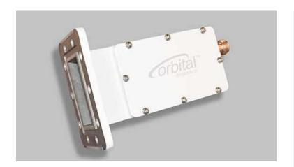
This external reference C-band LNB is enhanced to meet demanding specifications such as superior gain flatness, local oscillator (LO) stability and VSWR. It provides bandwidth of up to 800 MHz in the 3.40 to 4.20 GHz frequency range – and offers options like temperature-compensated gain and gain variations between 40 and 60 dB. This LNB is built for commercial and military SATCOM applications and is a great choice to help mitigate rain fade in temperate regions.
