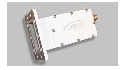
The Orbital 3300 C-Band Phase Locked Loop (PLL) LNB is a high-quality entry-level unit with good stability and noise temperature. It offers frequency ranges from 3.40 GHz to 4.20 GHz and bandwidth between 500 MHz and 800 MHz. Excellent gain flatness, a superior noise figure, and an economical price make this PLL LNB a perfect choice for traditional C-band applications like video – especially in rainy regions
