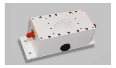
Built for airborne SATCOM and in-flight connectivity, these Ka-band block downconverters (BDCs) deliver market-leading performance and reliability in a ruggedized package. They come with either multiple or fixed local oscillators, provide bandwidth of up to 1 GHz, and can be tuned anywhere in the following Ka frequency bands: 18.2 to 20.2 GHz (option: 17.7 to 20.2 GHz) and 20.2 to 22.2 GHz. Like all
