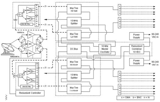
Due to unknown length, Orbital is unable to supply the cables shown as dashed lines. These cables are:
