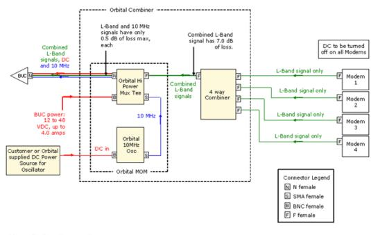
Orbital 4-way Combiner with 10 MHz Oscillator and hi power DC insert.
