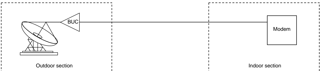
Figure 6: Simplified system diagram of a BUC transmit system.
