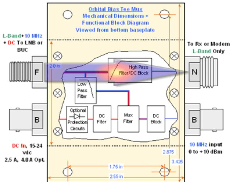
As a high pass filter and DC block for a receiver or modem.
