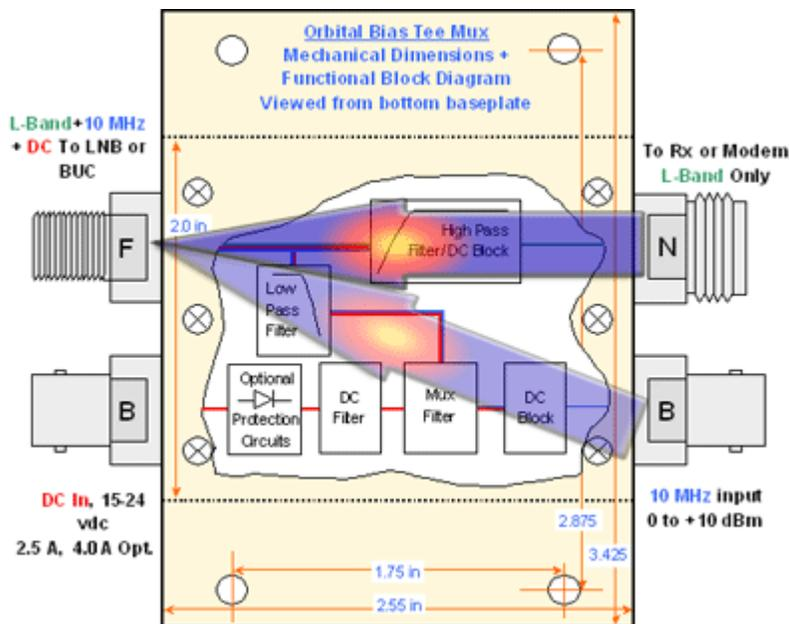
As a Diplexer to support a BUC, it becomes a System Interface Product (SIP), that combines a 10 MHz reference signal and L-Band output into one feed to a BUC. The **MT25/40 (as a Diplexer)** ensures low insertion loss, but high port-to-port isolation. Lock your BUC with the filtered diplexer. Puts the 10 MHz reference signal out to the BUC to lock it, and passes and filters the L-Band signal on the same line from the BUC.
