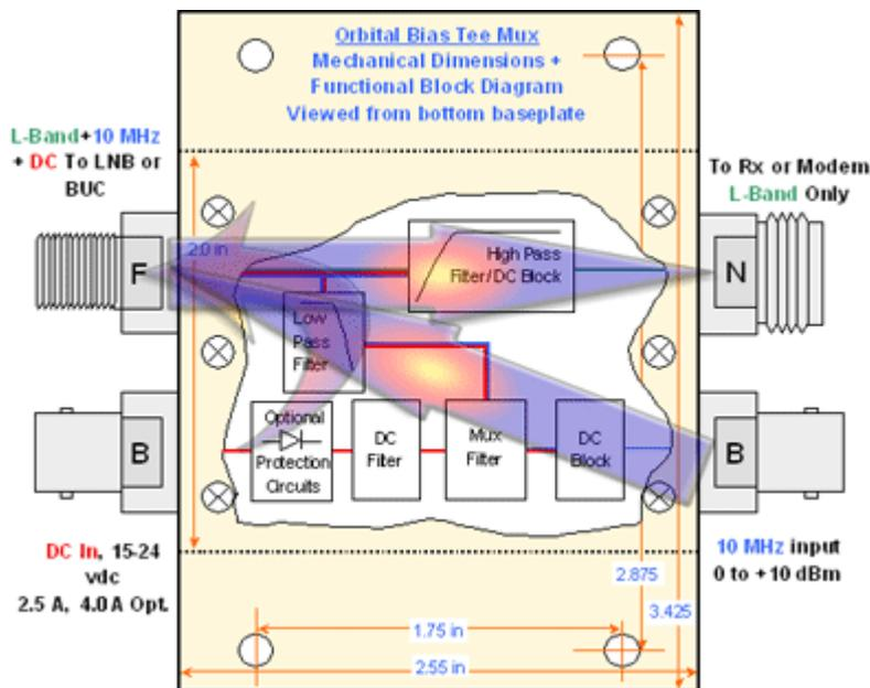
As a MuxTee the **MT25/40 Mux/Tee** integrates the L-band and DC filters of a *Bias Tee* with a 10 MHz Lowpass filter and an optional 20 MHz notch filter of a *Diplexer* to multiplex a 10 MHz external reference oscillator signal to your LNB or transmitter. What previously took a mixed bag of separate components is now available in an integrated bandpass-filtered and power-conditioned one-box solution ready for 'Back O Rack' mounting.
