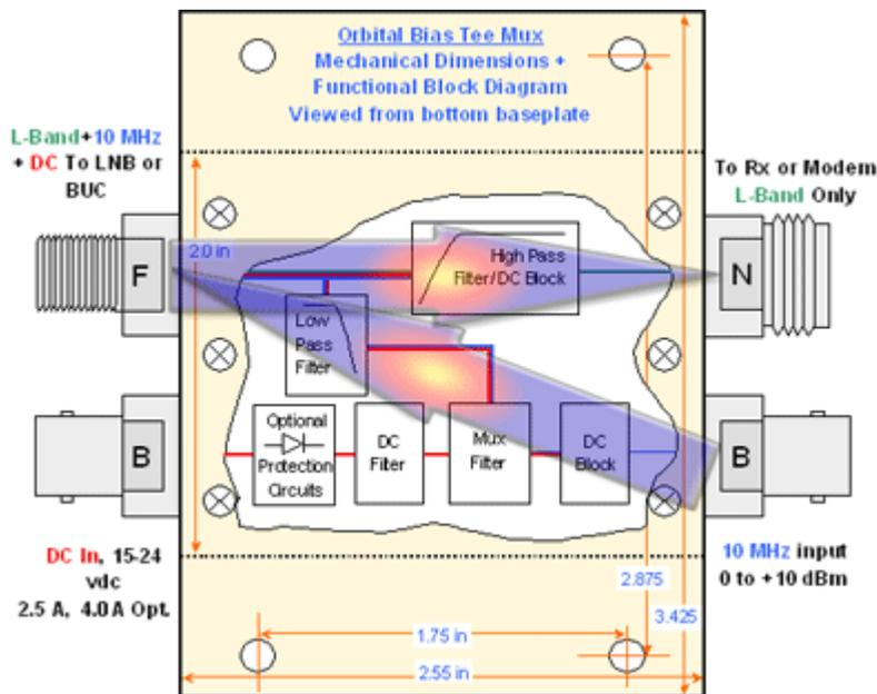
As a Diplexer to support a LNB, it becomes a System Interface Product (SIP), that combines a 10 MHz reference signal to an LNB, and L-Band output into one feed to a receiver. The **MT25/40 (as a Diplexer)**, ensures low insertion loss, but high port-to-port isolation. Lock your LNB with the filtered diplexer. Puts the 10 MHz reference signal out to the LNB to lock it, and passes and filters the L-Band signal on the same line from the LNB or to the receiver.
