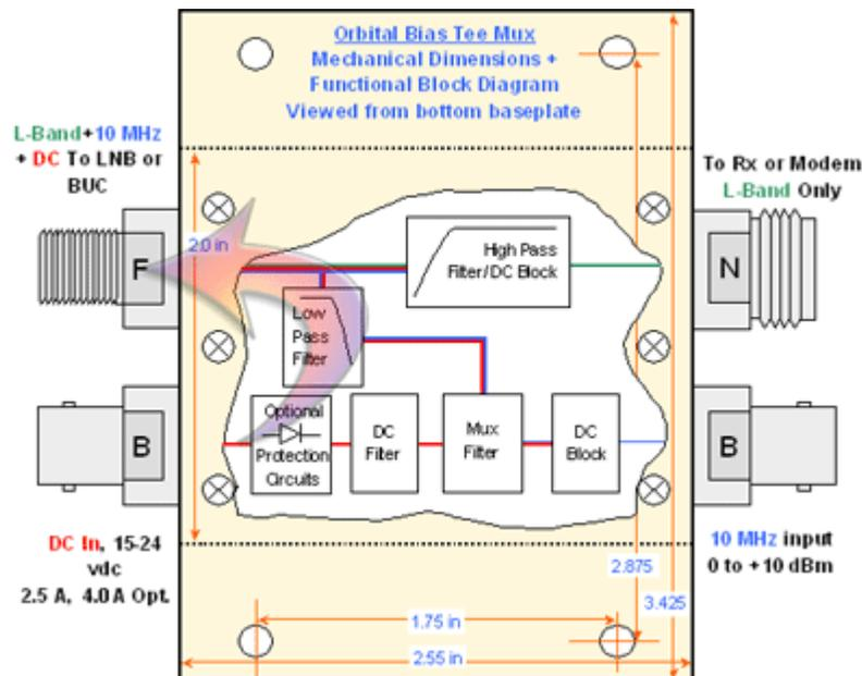
**As a Bias Tee, the MT25/40** injects and filters external DC to the LNB while providing exceptionally low thru loss and high-pass filtering of the L-band signal. What previously took a mixed bag of separate components is now available in an integrated bandpass-filtered and power-conditioned one-box solution ready for 'Back O Rack' mounting.
