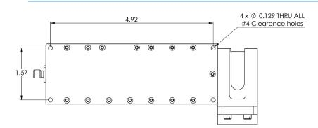
Connections J1: RF in (WR75-FBM, SQ. Grooved) J2: IF out, DC in &10M in (N female - 50ohm)
