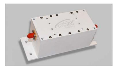
Our Ku-band block downconverters (BDCs) with fixed local oscillators (LOs) provide Ku coverage over ITU region 1, 2 or 3. We also have a wideband version that delivers full Ku spectrum coverage for mobile SATCOM applications. Standard LO frequencies are available and custom LOs can be provided to fit any application. These BDCs support high data throughput with very low bit error rates (BER).
